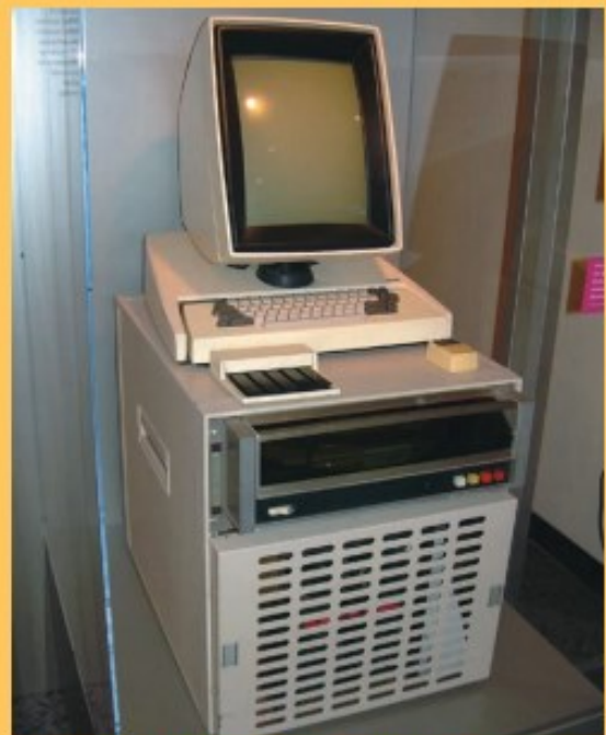
◆ Figure 3.2 The Xerox Alto was the first computer to use the desktop metaphor and the mouse-driven GUI. The separate hard drive seen below the computer could hold 2.5 megabytes (MB) of data.
