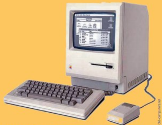
◆ Figure 3.1 The Macintosh computer was introduced in January 1984 and was the first to use a WIMP (windows, icons, menus and pointer) GUI.
